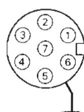
EXTERNAL VIEW OF CHASSIS CONNECTOR OR PLUG FROM THE SOLDERING SIDE
