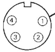
EXTERNAL VIEW OF CHASSIS CONNECTOR OR PLUG FROM THE SOLDERING SIDE
