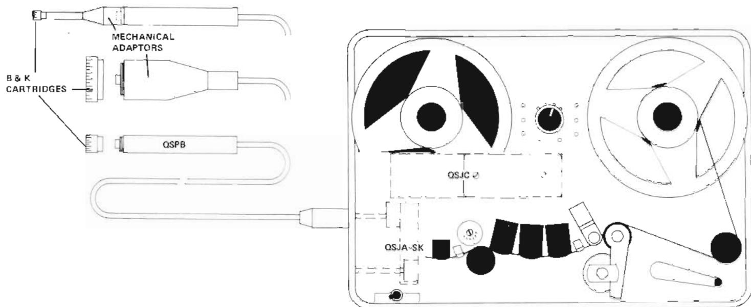
Brüel & Kjaer  $\frac{1}{2}$ " 4133, 4134, 4149 and 4163 microphone cartridges screw directly onto the QJPA preamplifier, and the preamplifier output plug fits into microphone connector 37. Other cartridges can be screwed on using a mechanical adapter, i.e.
