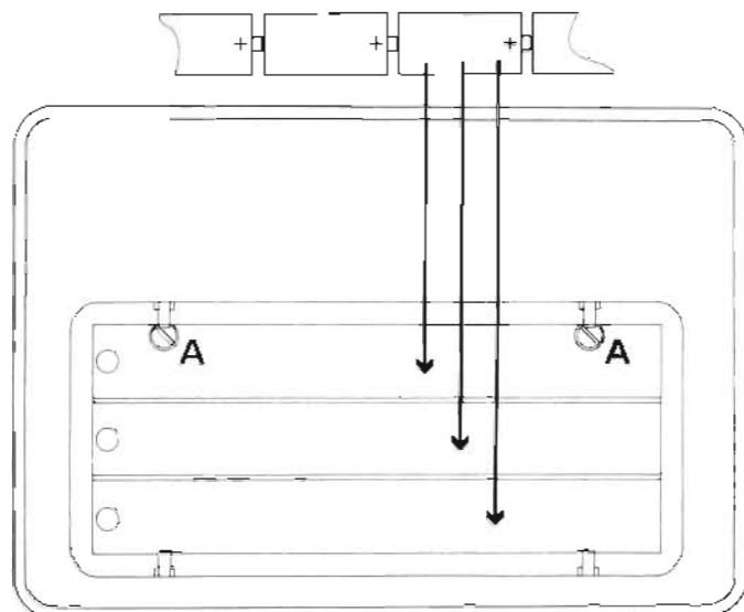
then replace the cover and secure it by turning the screws marked A. Set POWER switch 3 on Batt.
