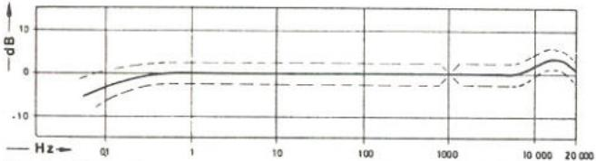
Standard frequency response with tolerance limits MKH 110-1.
