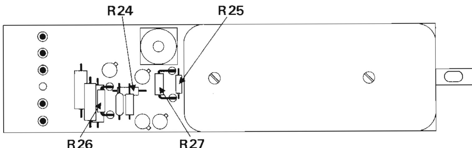
Version 1:  $R24 = 33 \text{ k}\Omega$ ,  $R25 = 27 \text{ k}\Omega$
