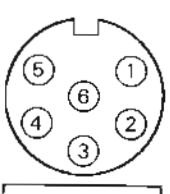
EXTERNAL VIEW OF CHASSIS CONNECTOR OR PLUG FROM THE SOLDERING SIDE
